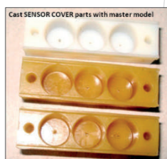
Figure 4 casted Sensor Cover parts master model.
